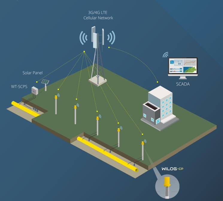
WILOG-CP is able to connect to Scada systems directly or via our NOVO Cloud Scada web service in order to send information for automatically adjusting the rectifiers required to achieve the perfect level of protection of the entire pipeline. Also, all alarms are sent in real time due to high/low or lack of protection level.
