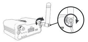
**1.** Connect the cellular antenna to the SMA connector. The correct way to install it is by screwing it clockwise.
