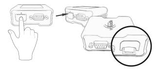
**2.** Insert the Micro Sim Card in the provided slot. Follow the guide to correctly insert it. The provided slot secures the Micro Sim Card to prevent it from disconnecting.
